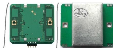
Gambar 1. Sensor radar HB100
